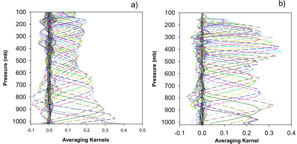
Fig. 1. Averaging kernels for temperature - **a)** and relative humidity - **b)** retrievals.
