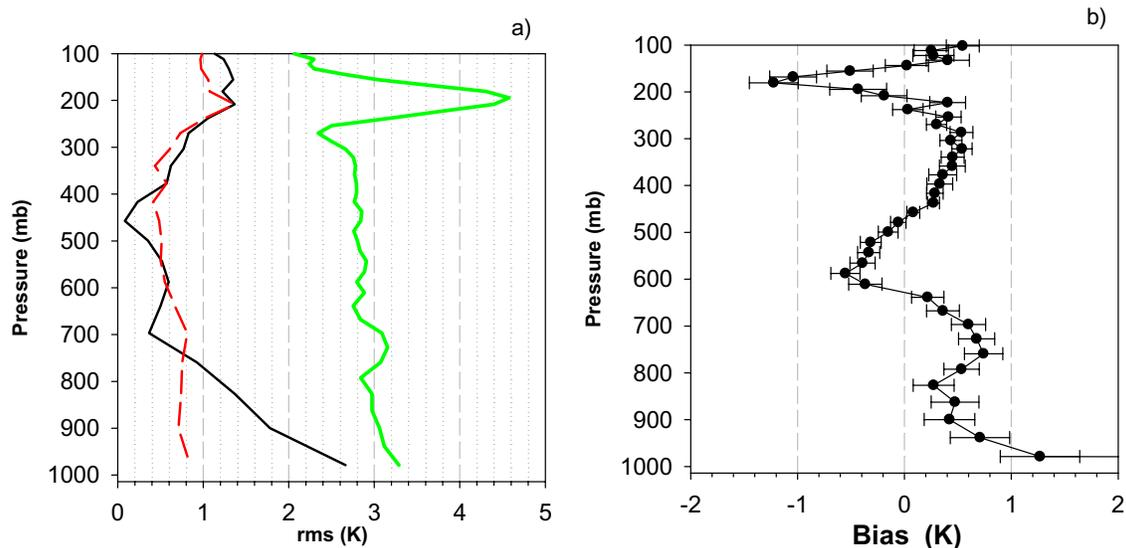
Fig. 3 Temperature. a) - Variances of: total retrieval error (assessed) - solid black line; total retrieval error (expected) - dashed red line; temperature profile - solid green line. b) Estimated bias against radiosondes.
