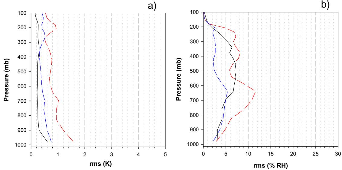
Fig. 2. Validation non-coincidence rms errors and noise for temperature - a) and relative humidity - b) retrievals. Variances (square roots of diagonal elements) of: temporal 0.5 hour non-coincidence - solid black line; effective 85 km spatial non-coincidence - red dashed line; and retrieval noise - blue dashed line.
