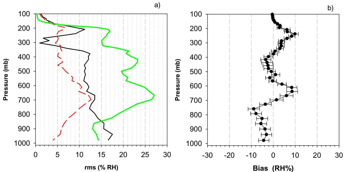
Fig. 4 Relative Humidity. a) - Variances of: total retrieval error (assessed) - solid black line; total retrieval error (expected) - dashed red line; relative humidity profile - solid green line. b) - Estimated bias against radiosondes.
